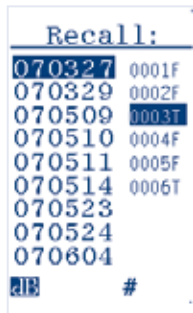
All measurements are stored using the actual date as current directory name
