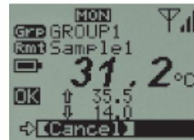
**Note:** If monitoring is carried out on a regular basis the battery life of the RTR-51,52,52Pt,53 units will be shortened. For example, if the monitoring interval is set at 1 minute the battery life will be about 4 months.
