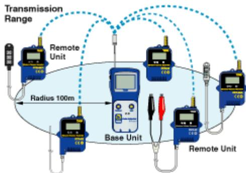
**Note:** If collecting data via wireless communication, it is necessary to register via computer the RTR-51,52, 52Pt,53 and RVR-52 as Remote Units and the RTR-57U as the Base Unit. The data recorded by the Remote Units can be downloaded via optical communication by placing it on the communication port of the RTR-57U.
